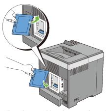
Close the control board cover and turn the screw clockwise.
